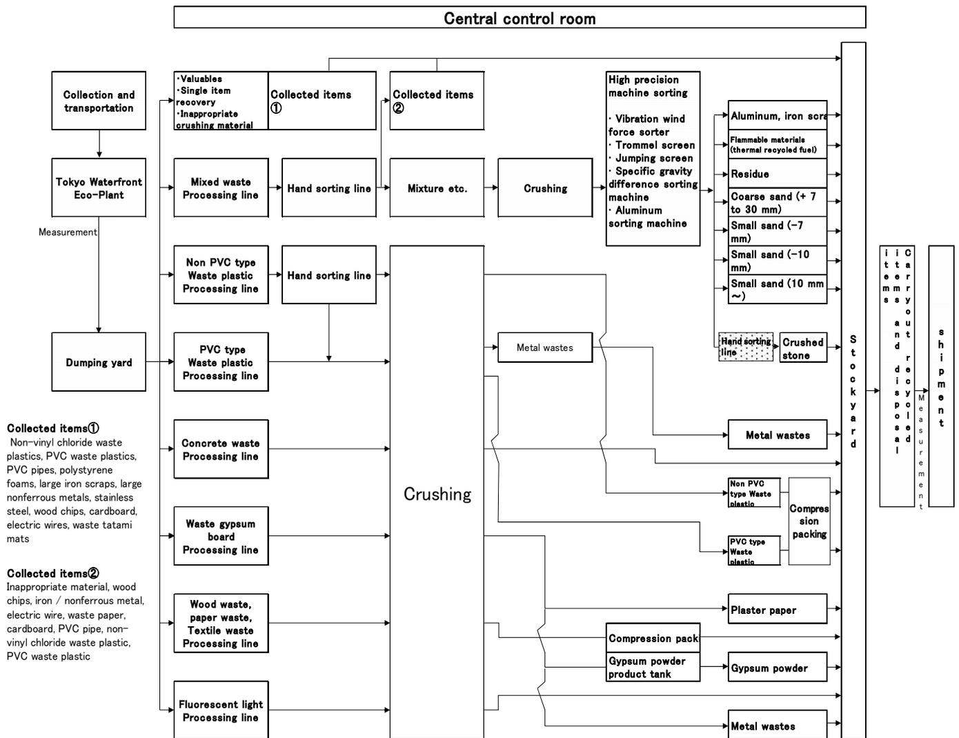
Figure 1 System flow of "High precision sorted recycling system"
