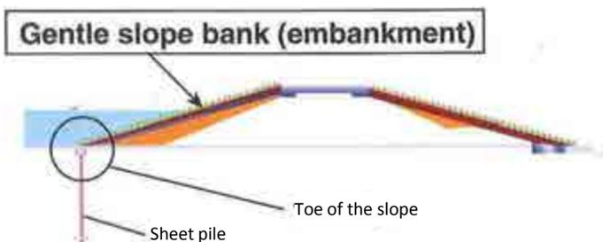
A gentle slope bank is build up by widening the bank cross-section. Increasing the bank cross-section makes a stable bank that is strong against floods. This method is used for draining quickly the water penetrated in the bank to lower the water level, by replacing soil around the toe of the slope on the river-back side (residence side) with permeable materials, such as stones.
