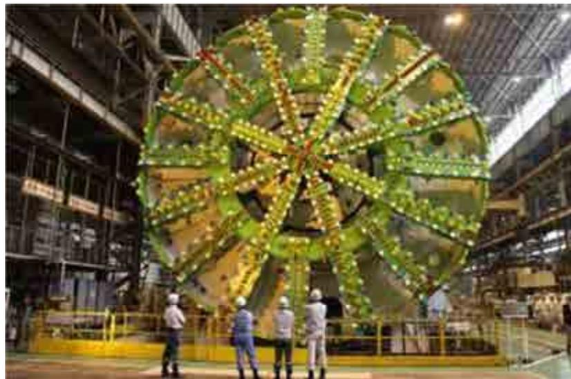
**Photo.1** Shielded machine with a diameter of about 16 m
