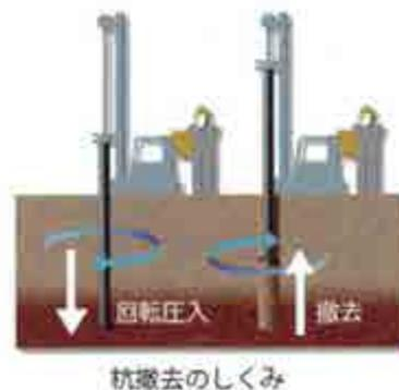
Figure 2 Structure of pile removal
