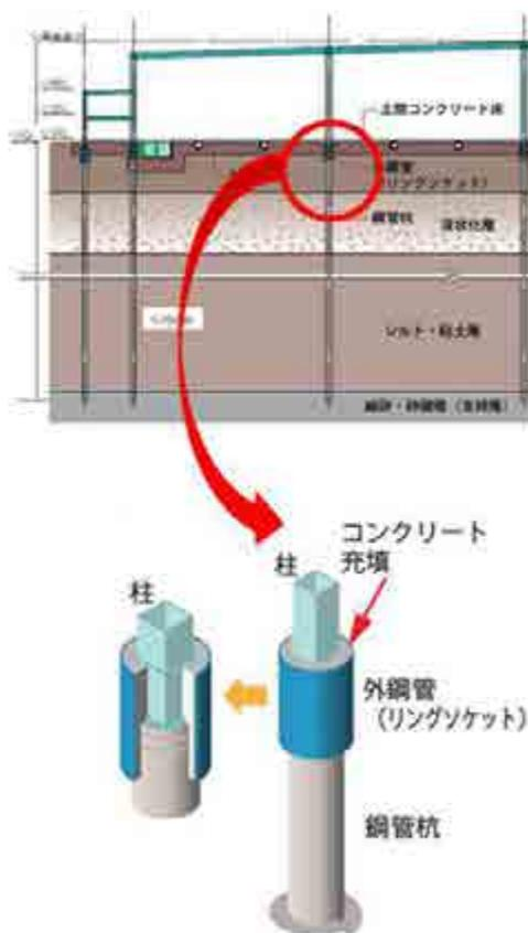
Figure 3 Sectional view of building and pile head ring socket
